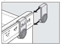
Slide the markers onto the guide runners on the edge of the drawers. Use the markers to indicate the type of food being frozen, and turn the dials to the appropriate number to indicate the month the food was first placed in the freezer.
